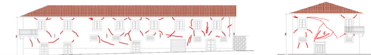
Figure 4. cracks detected on two external facades of the building
