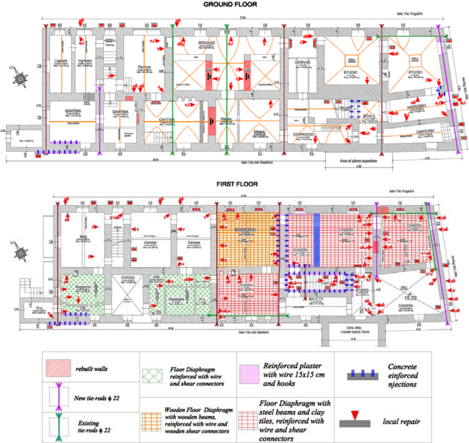
Figure 5: plans of interventions on the building,
